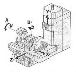
Figure Q2(a)(i): CNC Machine Configuration
