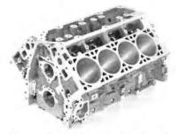
Figure Q1(a)(i): Engine Block
