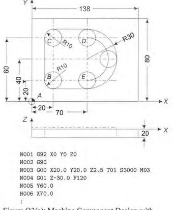
Figure Q3(c): Machine Component Design with Partial CNC Part Programming Coding
